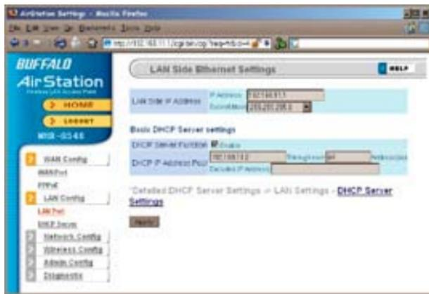
Default for the *LAN side IP address* is 192.168.11.1. To add the AirStation to an existing LAN, specify a unique IP address, not used elsewhere in the network.
