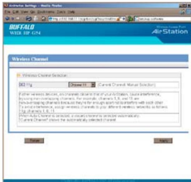
This page is available from *Home* by selecting *Wireless channel*. With *Auto Channel* selected, your AirStation will choose the best channel available. *Current channel* will show the channel that your AirStation is currently using.
