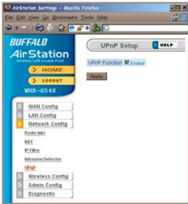
You may disable Universal Plug and Play functionality by unchecking *Enable* here. Note that Windows (MSN) Messenger will not function correctly with UPnP disabled.
