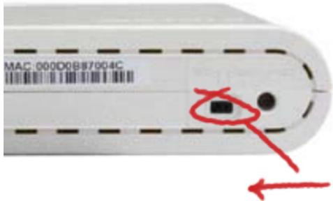
This AirStation supports quickly changing the product from a wireless router to a conventional access point.
