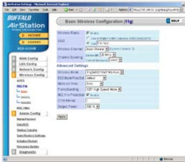
The SSID or network name can be changed by entering a custom SSID and pressing the Apply button.
