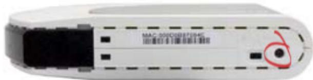
You may also initialize your AirStation by holding down the *Init* button on the bottom of the router for 3 seconds.
