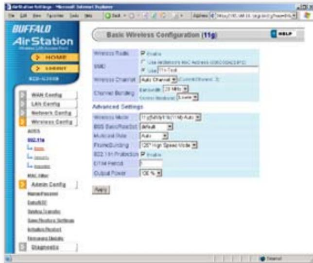
If you have a mixed mode network, with Draft-N, 802.11b and 802.11g clients, it's recommended that you check *11n protection* to ensure that slower 11b and 11g clients connect properly.
