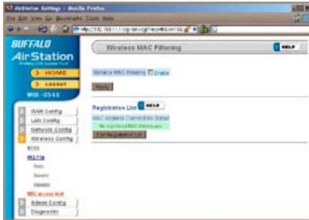
To setup a bridge between two or more wireless access points, select *Enable* and click on *Apply*.
