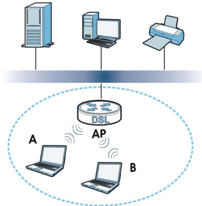
The wireless network is the part in the blue circle. In this wireless network, devices **A** and **B** are called wireless clients. The wireless clients use the access point (**AP**) to interact with other devices (such as the printer) or with the Internet. Your NBG-416N is the AP.
