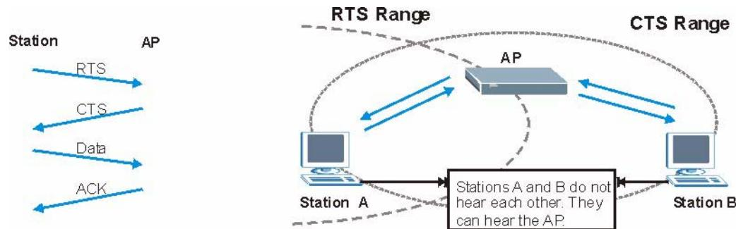
When station A sends data to the AP, it might not know that the station B is already using the channel. If these two stations send data at the same time, collisions may occur when both sets of data arrive at the AP at the same time, resulting in a loss of messages for both stations.
