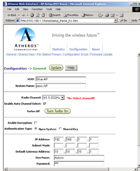
7. Enter the SSID (name or address) for the AP in the SSID field. The SSID must be 1-32 characters in length.
