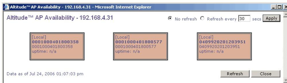
In normal operations, when the Summit WM series switch **Availability** feature is enabled, the local Altitude APs are green, and the foreign Altitude APs are red. If the other Summit WM series switch fails, and the foreign Altitude APs connect to the current Summit WM series switch, the display will show all Altitude APs as green. If the Altitude APs are not connected they show up as red.
