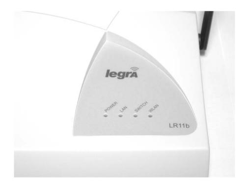
Figure 1-3 Legra Radio LEDs
