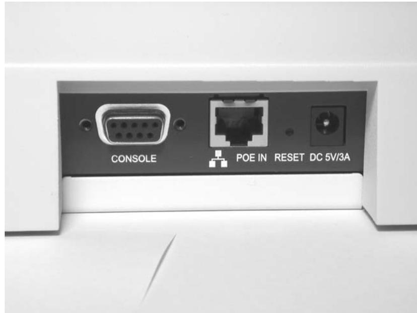
**Figure 1-2 Legra Radio Aft Connectors**
