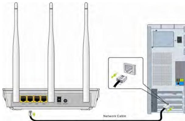
3. Connect the Ethernet cable from Internet side to the WAN port on the Device.
