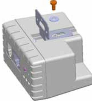
**Step 2 :** Slide the WAP-001 into the Bottom Faceplate and fasten tightly into the Bottom Faceplate until it's flushed into the wall.
