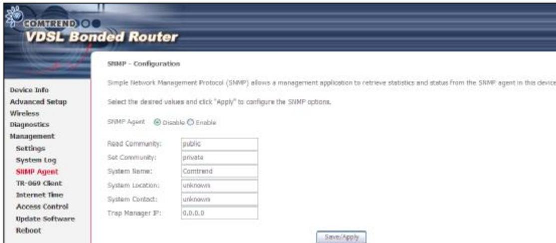
The screenshot shows the configuration page for the SNMP Agent on a COMTREND VDSL Bonded Router. The page title is "SNMP - Configuration". The left sidebar contains a menu with the following items: Device Info, Advanced Setup, Wireless, Diagnostics, Management, Settings, System Log, **SNMP Agent** (highlighted in red), TR-069 Client, Internet Time, Access Control, Update Software, and Reboot. The main content area contains the following text and form fields:
