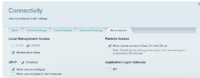
If your VoIP service uses SIP, select the SIP checkbox under *Application Layer Gateway*.
