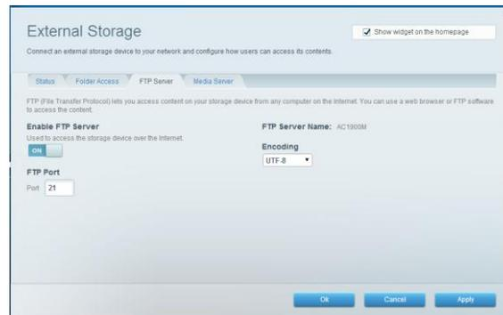
Toggle the switch for *Enable FTP Server* to turn it on.
