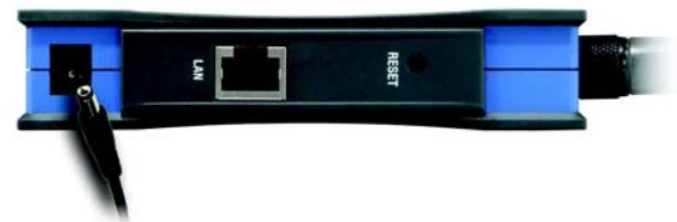
**Figure 4-2: Connect the Power**
