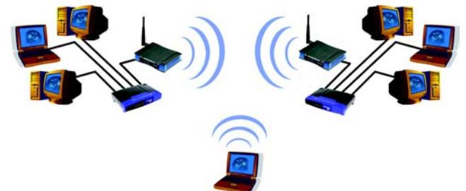
**Figure 2-3: Network Using Wireless Bridging**
