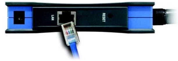
**Figure 4-1: Connect to the Network**
