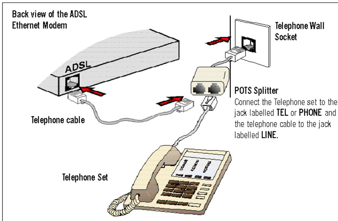
The POTS Splitter (with built-in Microfilter) is a device that allows you to connect both your Telephone cable and Telephone Set to the same Telephone Wall Socket. The device at the same time helps to eliminate background noise on the telephone line, ensuring the best possible phone performance.
