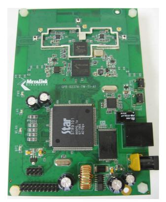
Figure 2-2 - MTW\_RGPLUS\_5.0\_VB\_001 Video Bridge board
