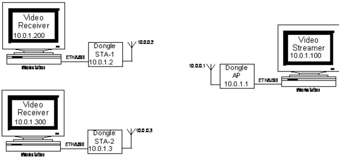
Figure 3-2 - Typical IP Assignment in Bridge mode
