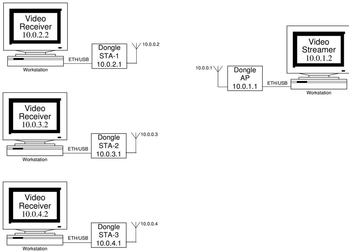
Figure 3-3 – Typical IP Assignment in route mode
