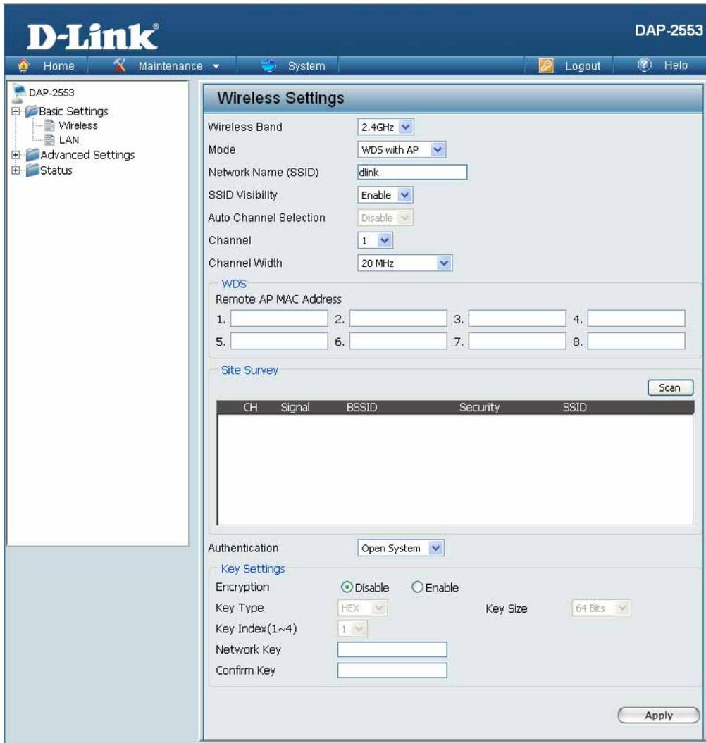
In WDS with AP mode, the DAP-2553 wirelessly connects multiple networks while still functioning as a wireless AP.
