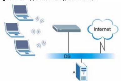
Figure 95 WPA(2) with RADIUS Application Example
