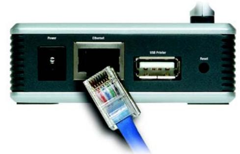
Figure 3-1: Connect to the Ethernet Port
