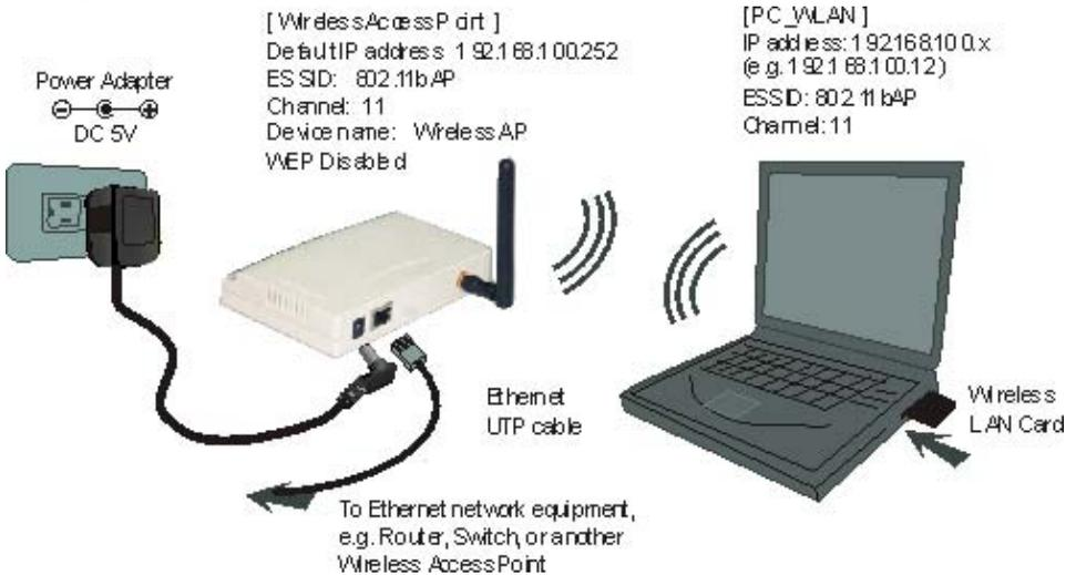
1. **Connect to your local area network:** connect an **Ethernet cable** to the **Ethernet** port of this Wireless Access Point, and the other end to a hub, switch, router, or another wireless access point.
