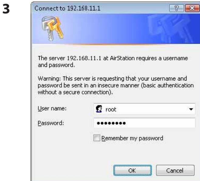
When this screen appears, enter "root" (in lower case) for the user name and the password that you set during initial setup. Click "OK".
