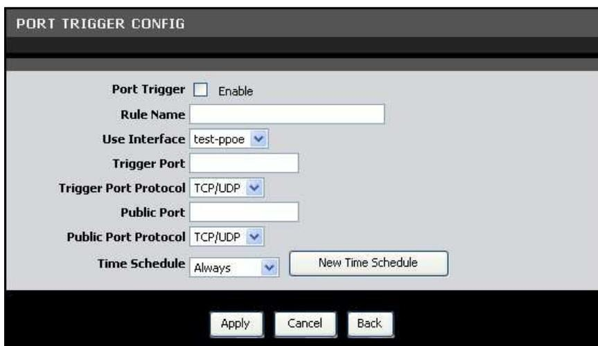
**Port Trigger** – Check this box to enable port triggering.
