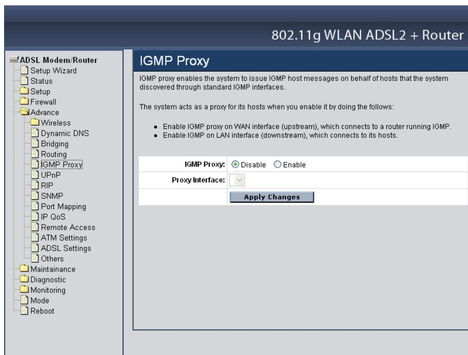
**IGMP Proxy:** Select to enable or disable the IGMP proxy feature on the WLAN ADSL Router.
