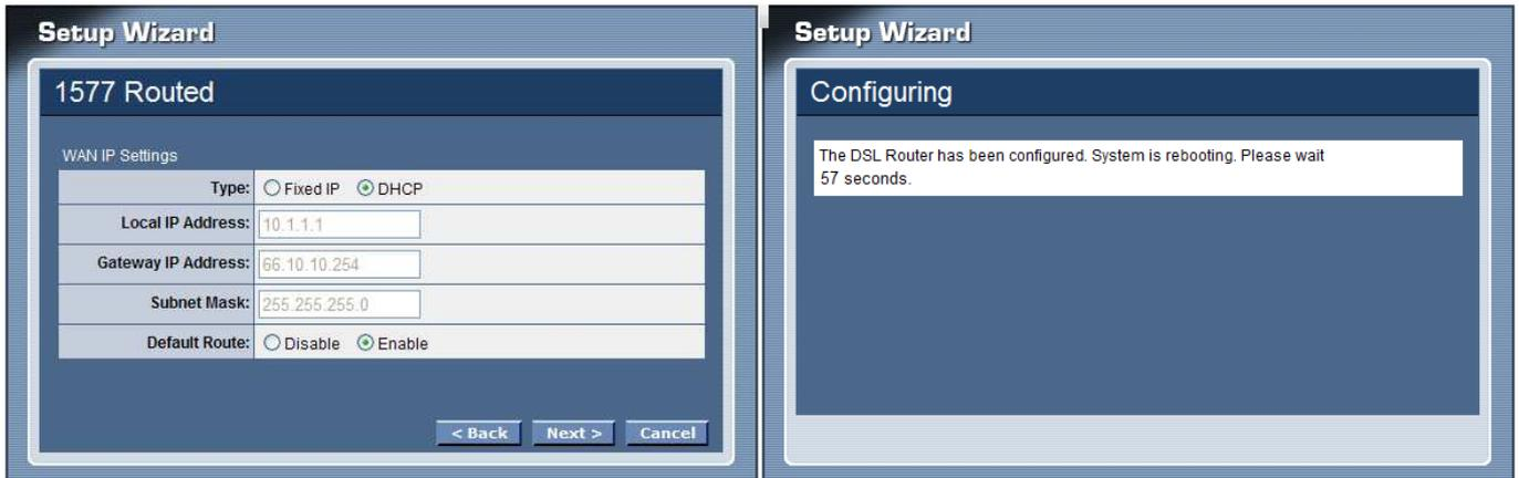
When rebooted the WLAN ADSL Router, enabled the “Test Internet Connection” then click finish button for test Internet connection; click close button close the setup wizard.
