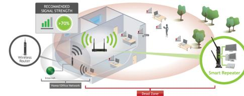
**IMPORTANT:** PLACE THE SMART REPEATER IN A LOCATION WHERE IT CAN RECEIVE A STRONG SIGNAL FROM YOUR WIRELESS ROUTER. This can be done before or after setup is complete. The Smart Repeater will save your settings.
