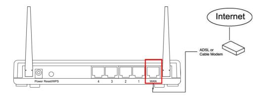
2. Connect all your computers, network devices (network-enabled consumer devices other than computers, like game console, or switch / hub) to the LAN port of the router.
