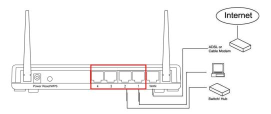
3. Connect the A/C power adapter to the wall socket, and then connect it to the 'Power' socket of the router.
