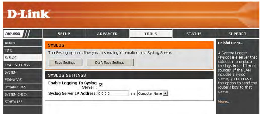
The screenshot displays the D-Link web management interface for the DIR-855L router. The top navigation bar includes the D-Link logo and tabs for SETUP, ADVANCED, TOOLS, STATUS, and SUPPORT. The left sidebar lists various configuration categories, with SYSLOG selected. The main content area is titled 'SYSLOG' and contains the following settings:
