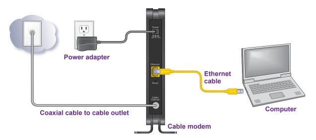
Figure 5. Connect the cable modem directly to a computer
