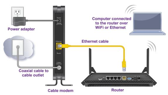
Figure 7. Connect the cable modem to a router
