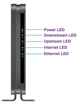
Figure 2. Cable modem front view
