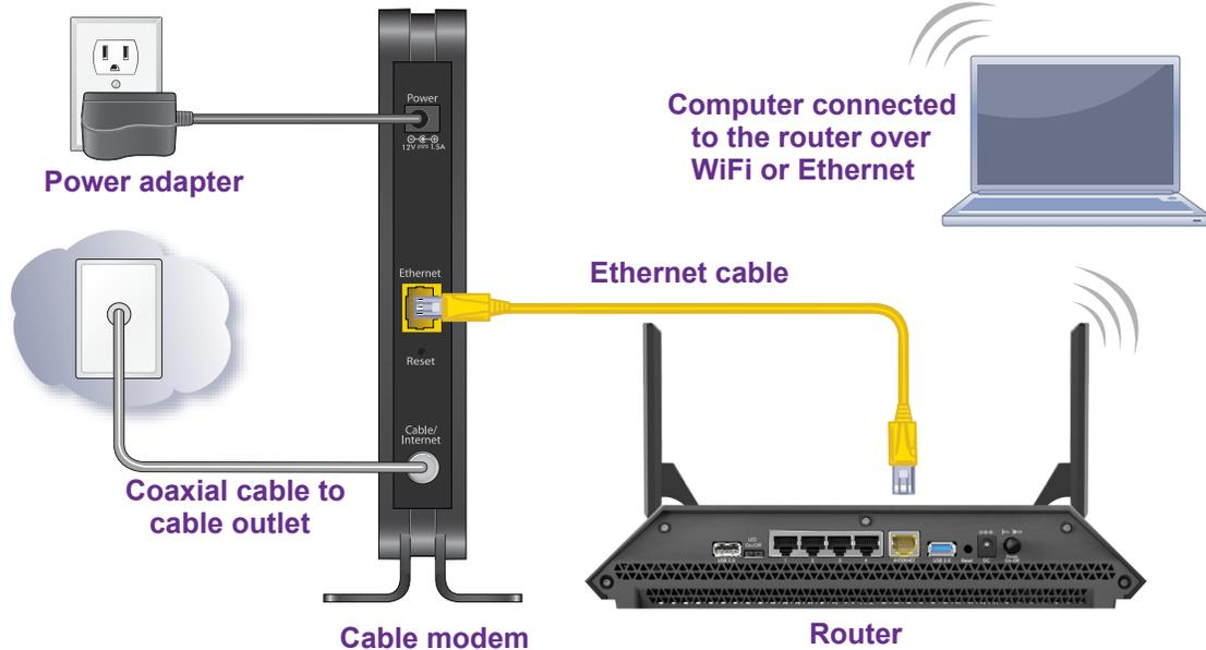
Figure 7. Connect the cable modem to a router
