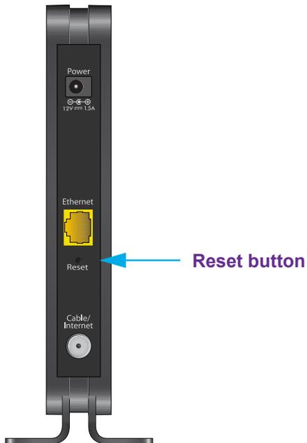
3. Using a straightened paper clip, press and hold the **Reset** button for about seven seconds until all LEDs blink.
