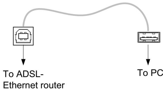
Figure 85: USB Cable Connectors
