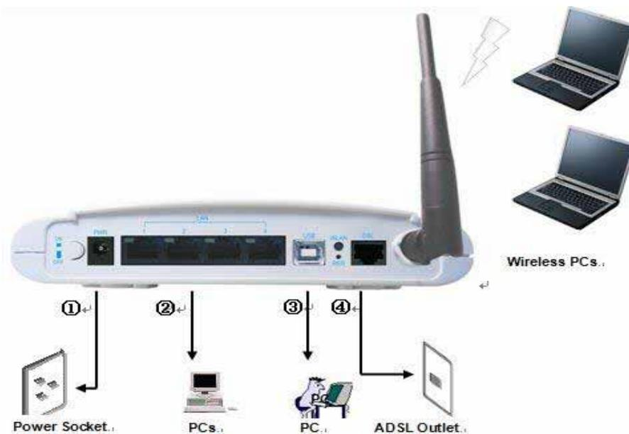
**Figure 8: Overview of Hardware Connections for X7967r**
