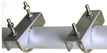
Next, attach the plate, using two nuts, as shown in Figure 12. Adjust the nuts to insure that the U-bolts do not protrude past the fold in the plate. The exact adjustment depends on pole diameter.
