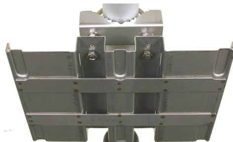
When the plate is mounted and aligned, tighten all the nuts with a 7/16-inch wrench. Next, slide the HotPoint onto and downward slightly, so that its tabs on its backing plate (Figure 13) engage the mounting plate, as shown in Figure 13. Tighten the four knurled nuts on the sides.
