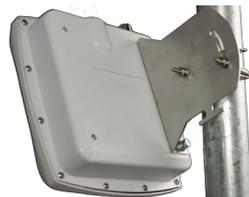
The Firetide HotPoint 4200 requires power. Power is fed via Ethernet. Connect the power-feed unit to AC power. The ON light should turn green. Plug the cable from the HotPoint into the port marked OUT. The CONNECT light should turn green. If the FAULT light comes on, contact Firetide.
