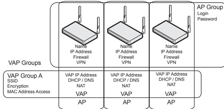
Figure 16 shows a three-AP, three-VAP configuration. You can have multiple VAPs per physical AP.
