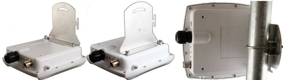
The bracket is attached to the pole using the U-bolt and one or two of the supplied jaw-clamps (top left in Figure 4). One jaw-clamp is used between the bracket and the pole; the second clamp may be used on smaller-diameter poles by placing it over the U-bolt before putting the U-bolt around the pole.
