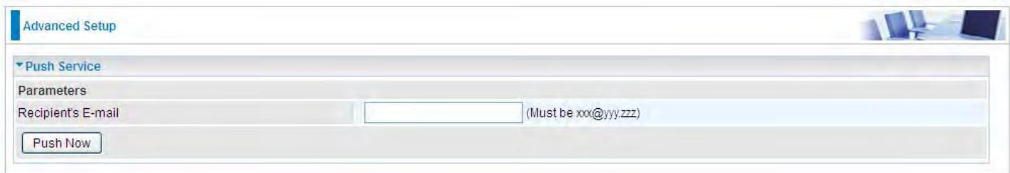
**Recipient's E-mail:** Enter the destination mail address. The email is used to receive **system log**, **system configuration**, **security log** sent by the device when the **Push Now** button is pressed (information sent only when pressing the button ), but the mail address is not remembered.
