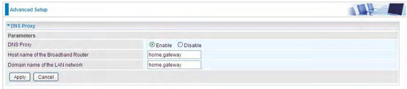
**DNS Proxy:** Select whether to enable or disable DNS Proxy function, default is enabled.
