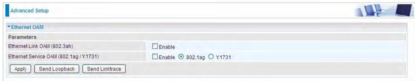
**Ethernet Link OAM(802.3ah):** Enable to activate Ethernet in the First Mile (EFM) Link OAM to do link fault management.
