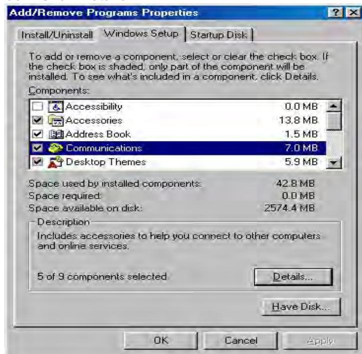
**Step 3:** In the Communications window, select the Universal Plug and Play check box in the Components selection box.
