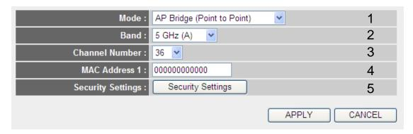
NOTE: Two wireless routers must use the same mode, band, channel number, and security setting!
