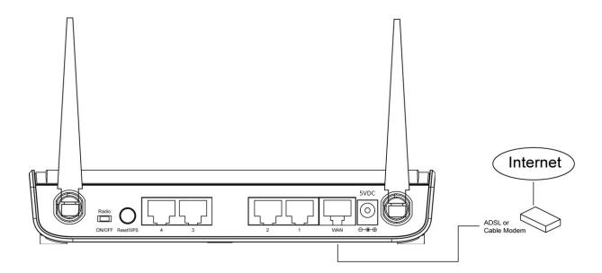
2. Connect all your computers, network devices (network-enabled consumer devices other than computers, like Game console, or Switch / Hub) to the LAN port of the router.
