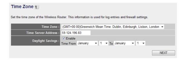
Please select time zone at 'Time Zone' drop-down list, and input the IP address or host name of time server. If you want to enable daylight savings setting, please check 'Enable' box, and set the duration of daylight setting. When you finish, click 'Apply'. You'll see the following message displayed on web browser:
