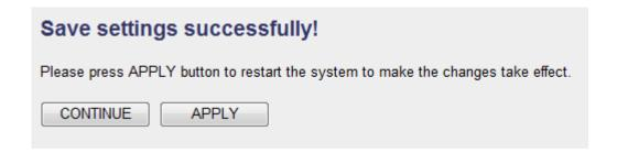
Press 'Continue' to save the settings made and back to web management interface; press 'Apply' to save the settings made and restart the router so the settings will take effect after it reboots.
