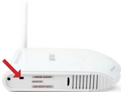
This AirStation supports quickly changing the product from a wireless router to a conventional access point.
