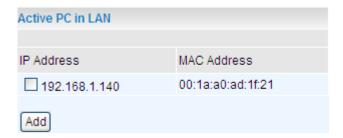
**Active PC in LAN:** Active PC in LAN window displays a list of IP Address & MAC Address of each Ethernet device which connects to the router.
