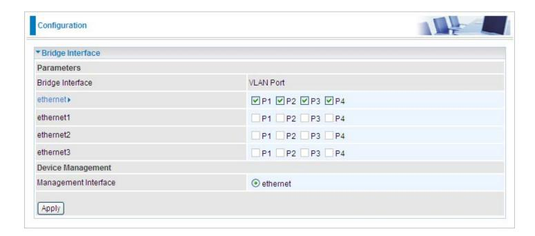
You can setup member ports for each VLAN group under Bridge Interface section. From the example, two VLAN groups need to be created.
