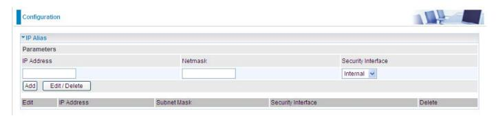
**IP Address:** Specify an IP address for this virtual interface.
