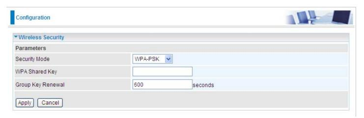
**Security Mode:** You can disable or enable with WPA or WEP for protecting wireless network. The default mode of wireless security is **Disable**.
