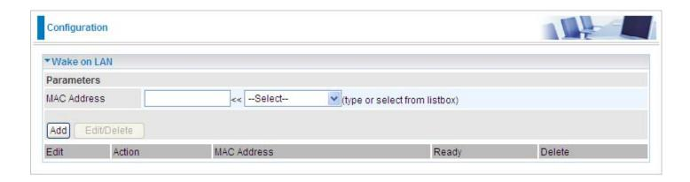
**MAC Address:** Enter the MAC address of the target computer or you can select the MAC address directly from the Select drop down menu on the right.
