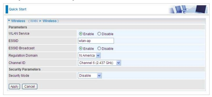
**WLAN Service:** Default setting is set to **Enable**. If you want to use wireless, both 802.11g and 802.11b device in your network, you can select **Enable**.
