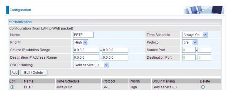
The mission-critical application must be sent out smoothly without any drop out. Set the level of priority as high to prevent other applications from saturating the bandwidth.
