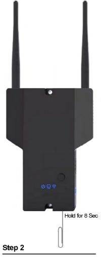
Using a paper clip, press and hold the reset button located on the bottom of the MV2458 for approximately 8 seconds and then let go.
