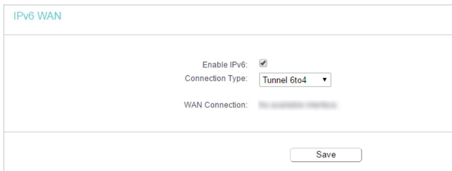
The screenshot shows the 'IPv6 WAN' configuration interface. It includes a title bar 'IPv6 WAN', a 'Save' button at the bottom right, and three configuration fields: 'Enable IPv6' with a checked checkbox, 'Connection Type' with a dropdown menu set to 'Tunnel 6to4', and 'WAN Connection' with a blurred selection.
