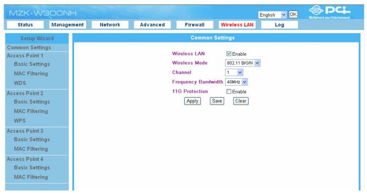
MZK-W300NH can simulate four different Access Points (APs), so you can have four different APs with different settings. You can configure these four access points by clicking the "**Wireless LAN**" tag on the upper part of the webpage.
