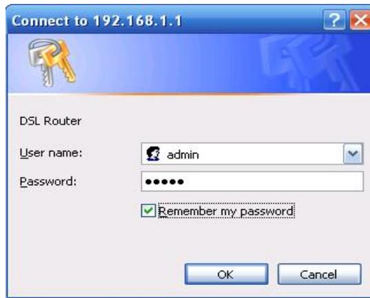
After logging in to the DSL router as a super user, you can query, configure, and modify all configurations, and diagnose the system.
