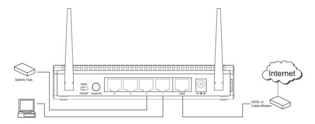
3. Connect the A/C power adapter to the wall socket, and then connect it to the 'Power' socket of the router.
