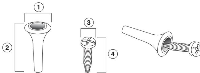
**1** 8 mm/0.31 in    **2** 25 mm/0.98 in    **3** 6.5 mm/0.26 in    **4** 17.9 mm/0.7 in
