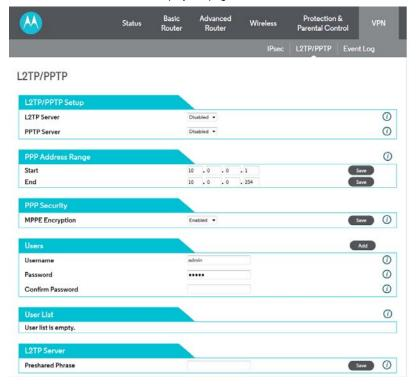
Figure 41 L2TP/PPTP configuration
