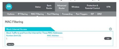
Figure 20 MAC Filtering configuration
