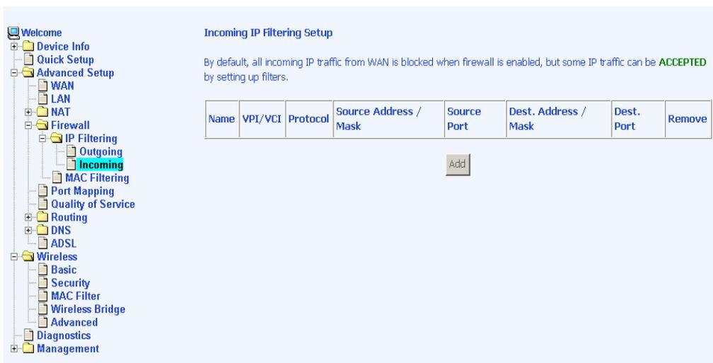
Enter a filter name, information about the source address (from the WAN side), and information about the destination address (to the LAN side). Select the protocol and WAN interface, then click on **Save/Apply** to add the setting.
