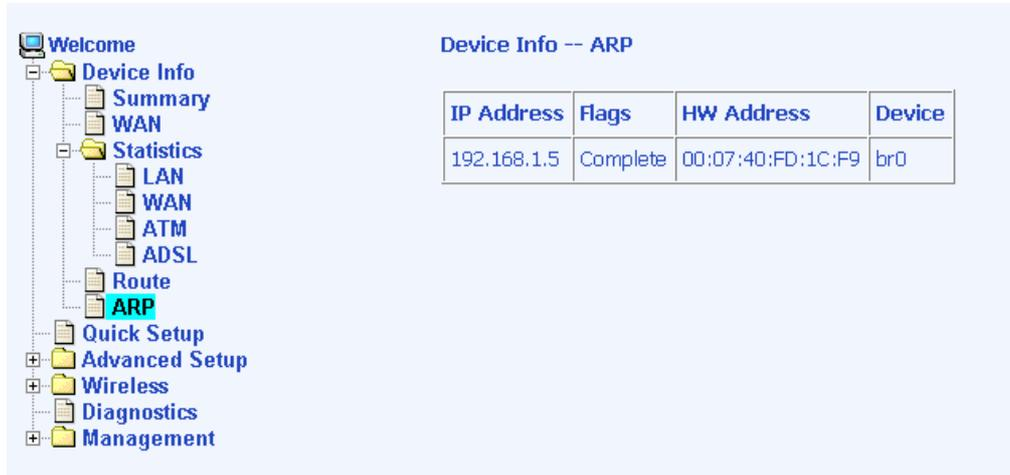
The screenshot displays the router's web interface. On the left is a navigation tree with the following items: Welcome, Device Info (expanded), Summary, WAN, Statistics (expanded), LAN, WAN, ATM, ADSL, Route, ARP (highlighted in red), Quick Setup, Advanced Setup, Wireless, Diagnostics, and Management. On the right, the page title is "Device Info -- ARP" and a table shows the ARP entry for interface br0.
