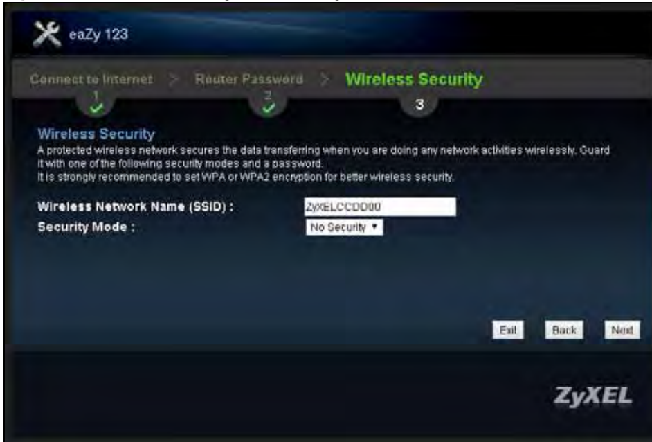
Figure 13 Wireless Security: No Security
