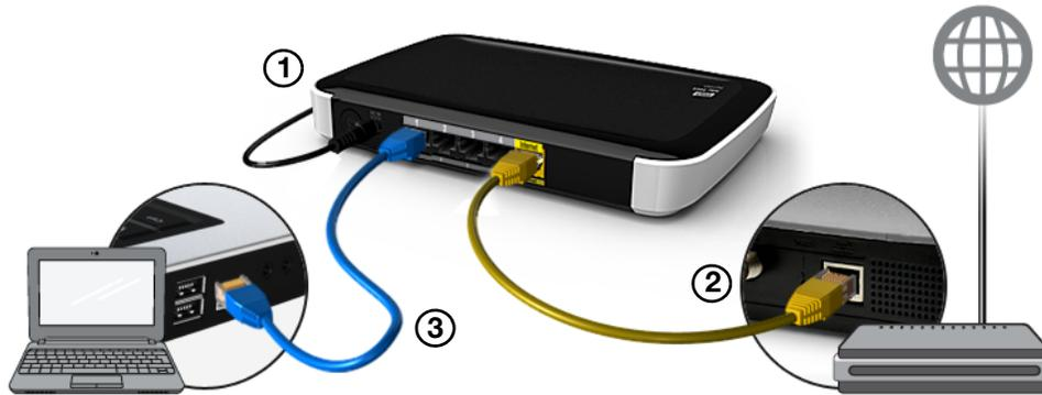
1. Connect the power cable to the router's DC connector and into an AC power outlet. Press the **On/Off** button on the back of the router once to turn it on. The four LEDs on the front the router light up one by one as it boots up.
