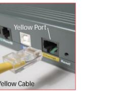
**Step 7** Plug one end of the **Yellow Cable** into the **Yellow Port** on the back of the Wireless DSL Gateway.
