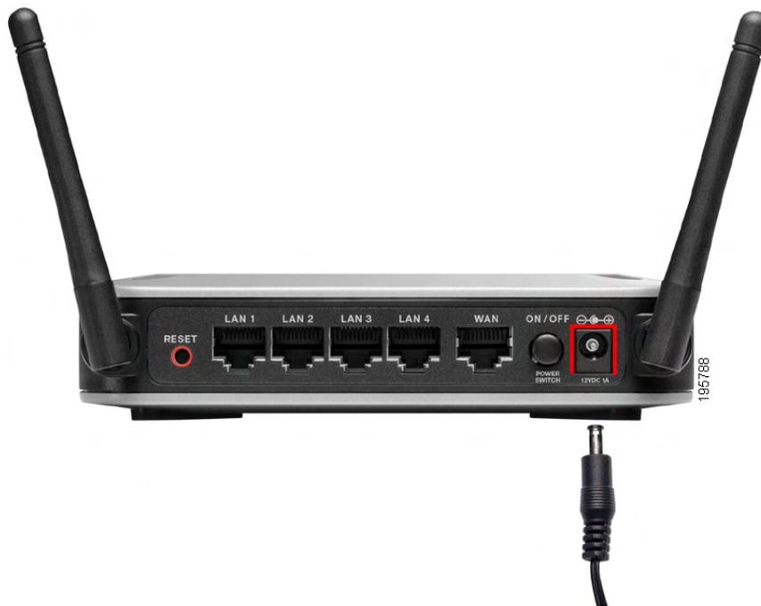
**STEP 5** Plug the other end of the adapter into an electrical outlet.
