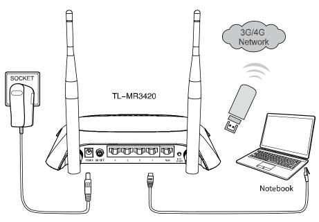
Figure 2-1 Hardware Installation – 3G/4G connection
