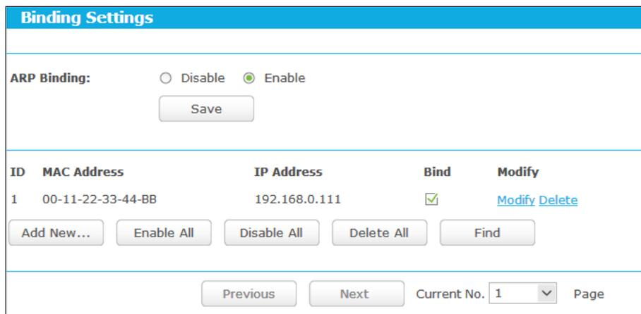
Figure 5-69 Binding Setting
