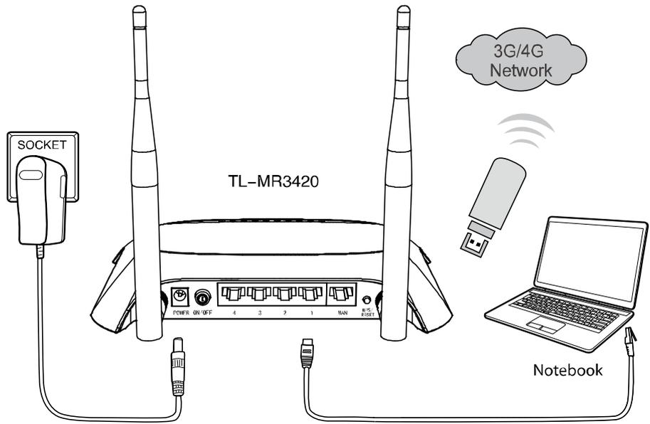
Figure 2-1 Hardware Installation – 3G/4G connection
