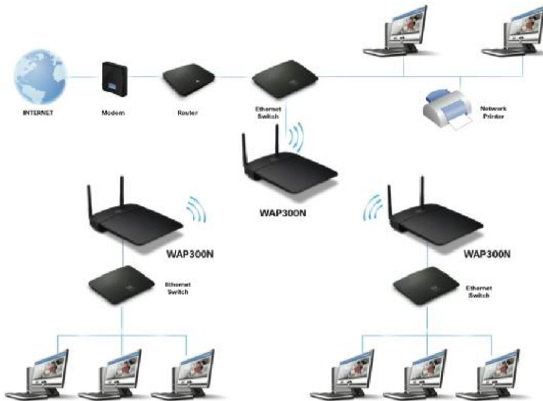
With multiple WAP300Ns operating in this mode, WAP300Ns can wirelessly connect two or more wired networks together.
