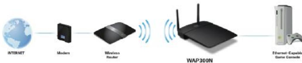
In this mode, WAP300N adds wireless networking capability to any wired (Ethernet-capable) device (e.g. game console, media player, DVR, smart TV or network access storage). If you have a wired network device, connect it to this device for wireless network access.
