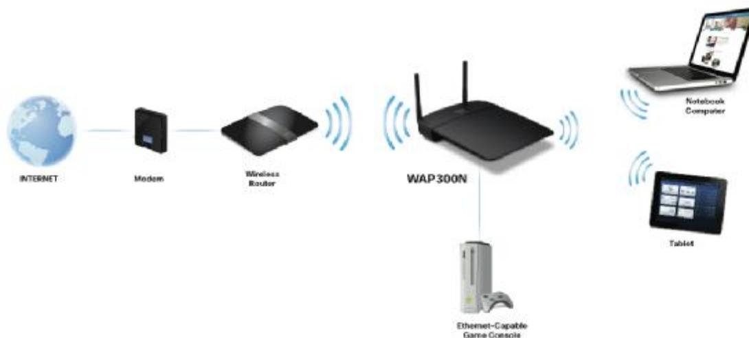
In this mode, this device wirelessly extends the range of an existing wireless network. At the same time, it also adds wireless networking capability to any wired (Ethernet-capable) device (e.g. game console, media player, DVR, smart TV or network access storage).
