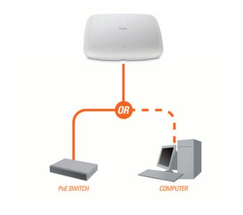
Connect one end of an Ethernet cable (included with your access point) to the LAN port on the DAP-2320 and the other end of the Ethernet cable to either your computer or to your PoE switch. The AP can be powered on by a PoE switch or by the power adapter shipped with the AP.
