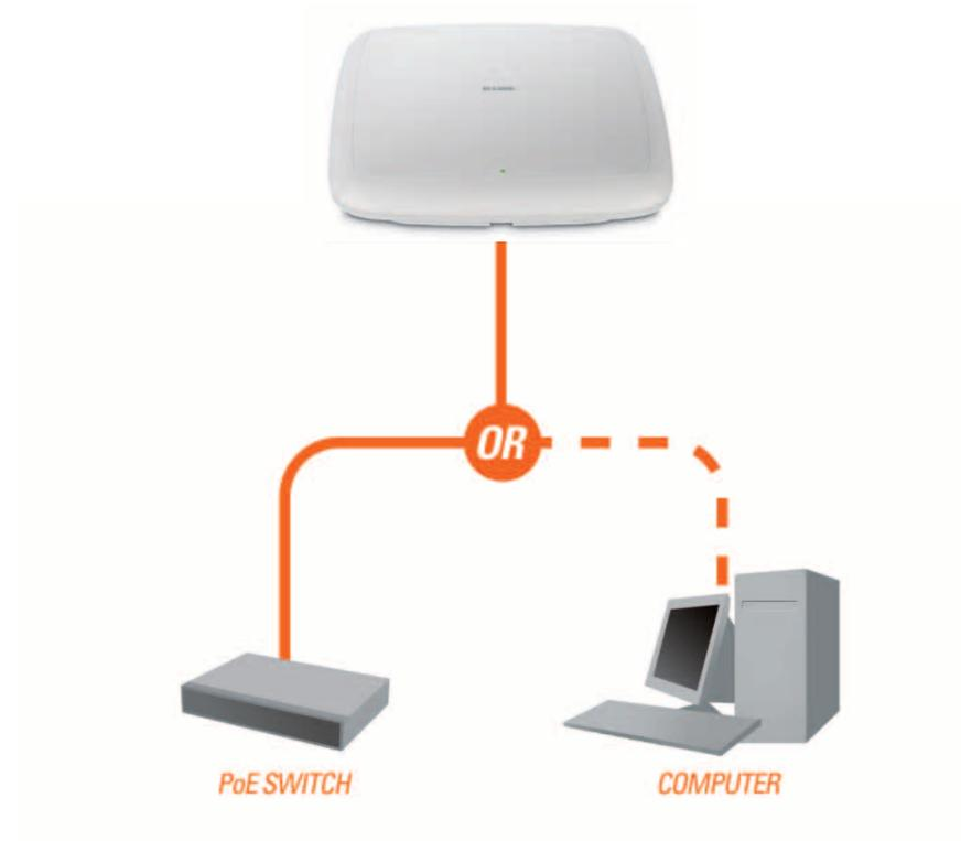
Connect one end of an Ethernet cable (included with your access point) to the LAN port on the DAP-2320 and the other end of the Ethernet cable to either your computer or to your PoE switch. The AP can be powered on by a PoE switch or by the power adapter shipped with the AP.
