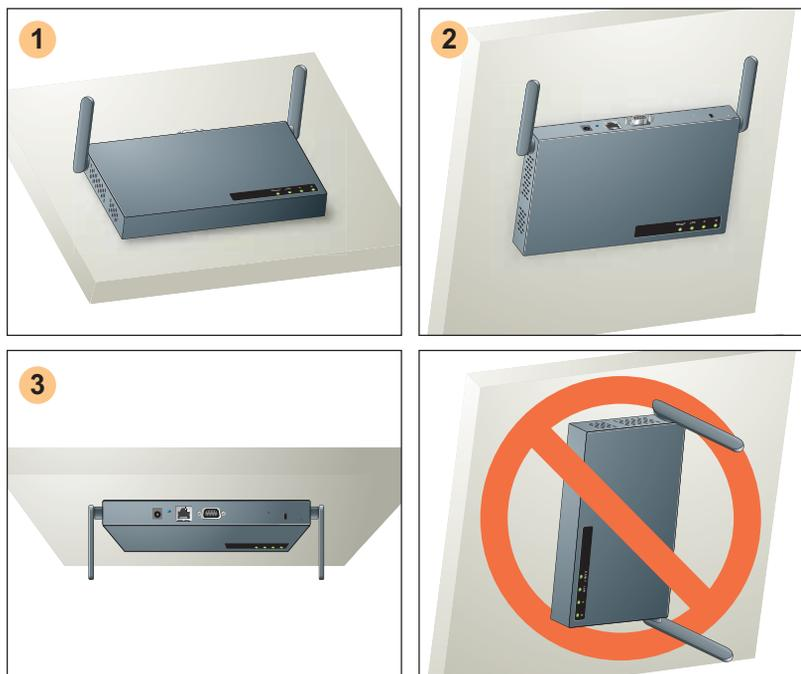
FIGURE 2-2 Aruba 52 Mounting Options
